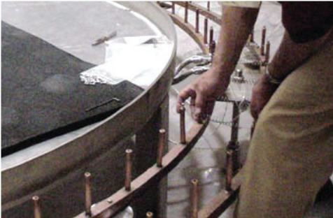
Posts along electrically conductive rings at bottom of coating tank. Tungsten filaments stretched across these posts will be heated to incandescence until aluminum strands tied along the filaments evaporate.
